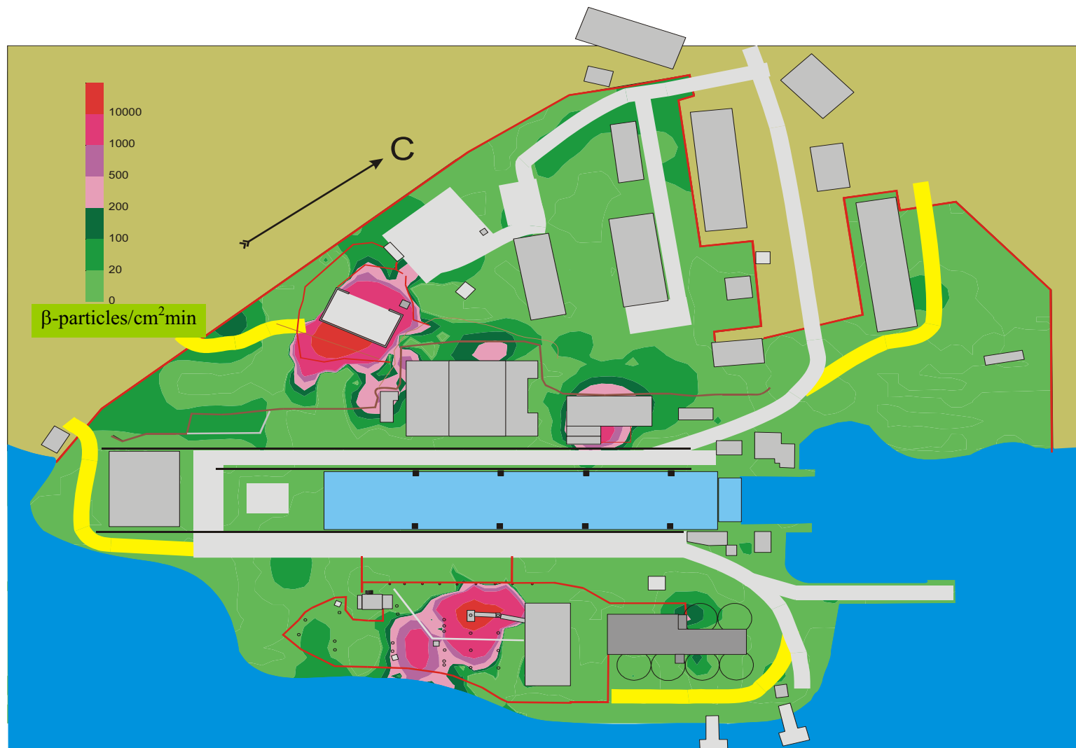
Fig. 4b. Density of \beta -radiation flux on the RW and SNF TSF territory in Gremikha
