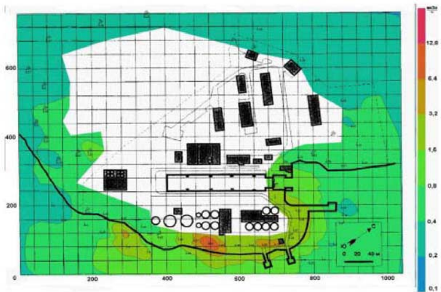
Cartogram of the Dose Rate at the Height of 1 m at the Coastline and along the Site Outer Perimeter
