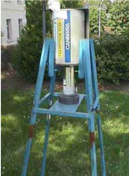
In situ gamma spectrometry for soil/site characterization
