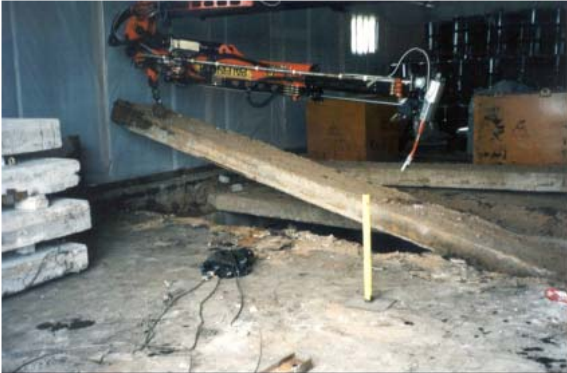
Fig. 25. The main crane with jib and gamma probe
