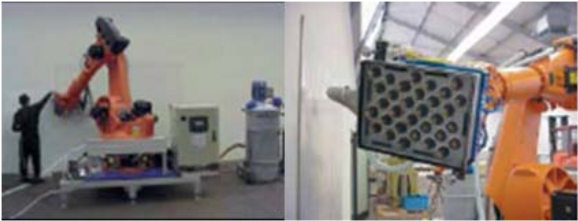
Fig. 44. Decontamination robot, BOLERO, from Studsvik SINA
