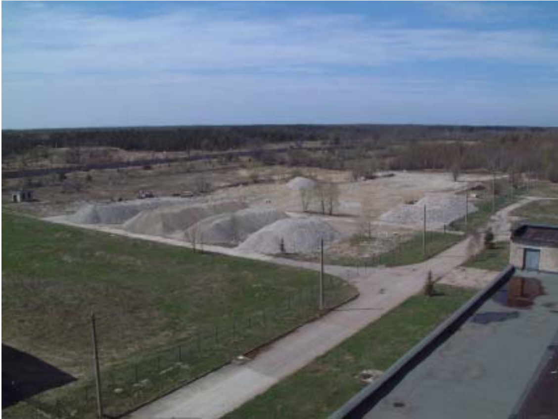
Fig. 46. Piles of crushed concrete.
