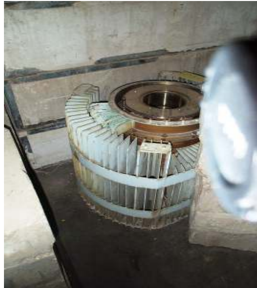
Fig 1b) A typical RTG ( ^{90}\text{Sr} heat source removed)
