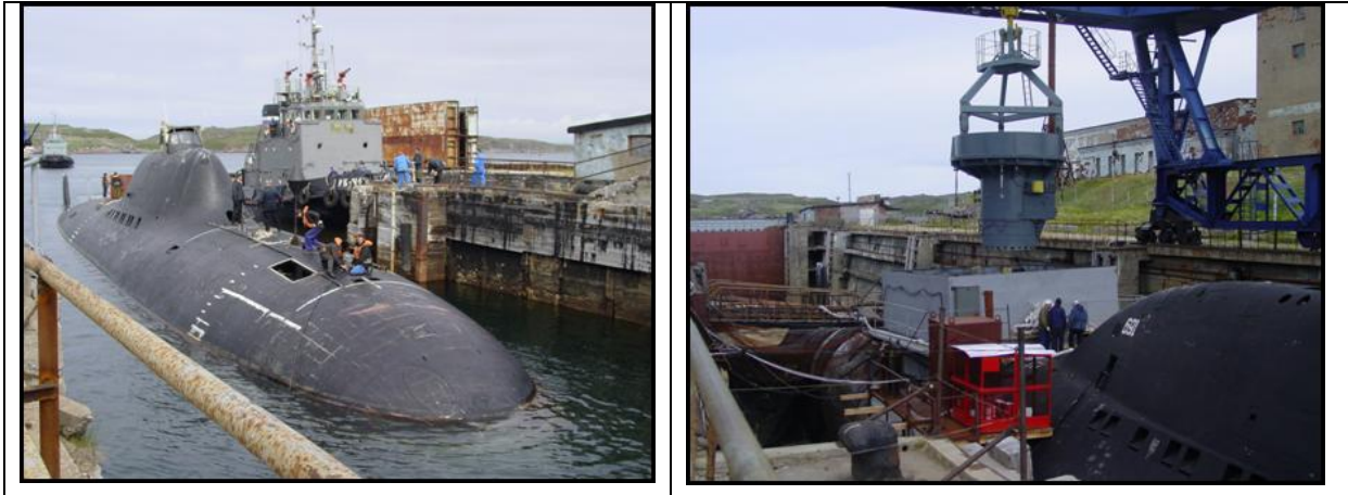
Figure 1. Preparation of the Alfa-class submarine for defuelling
