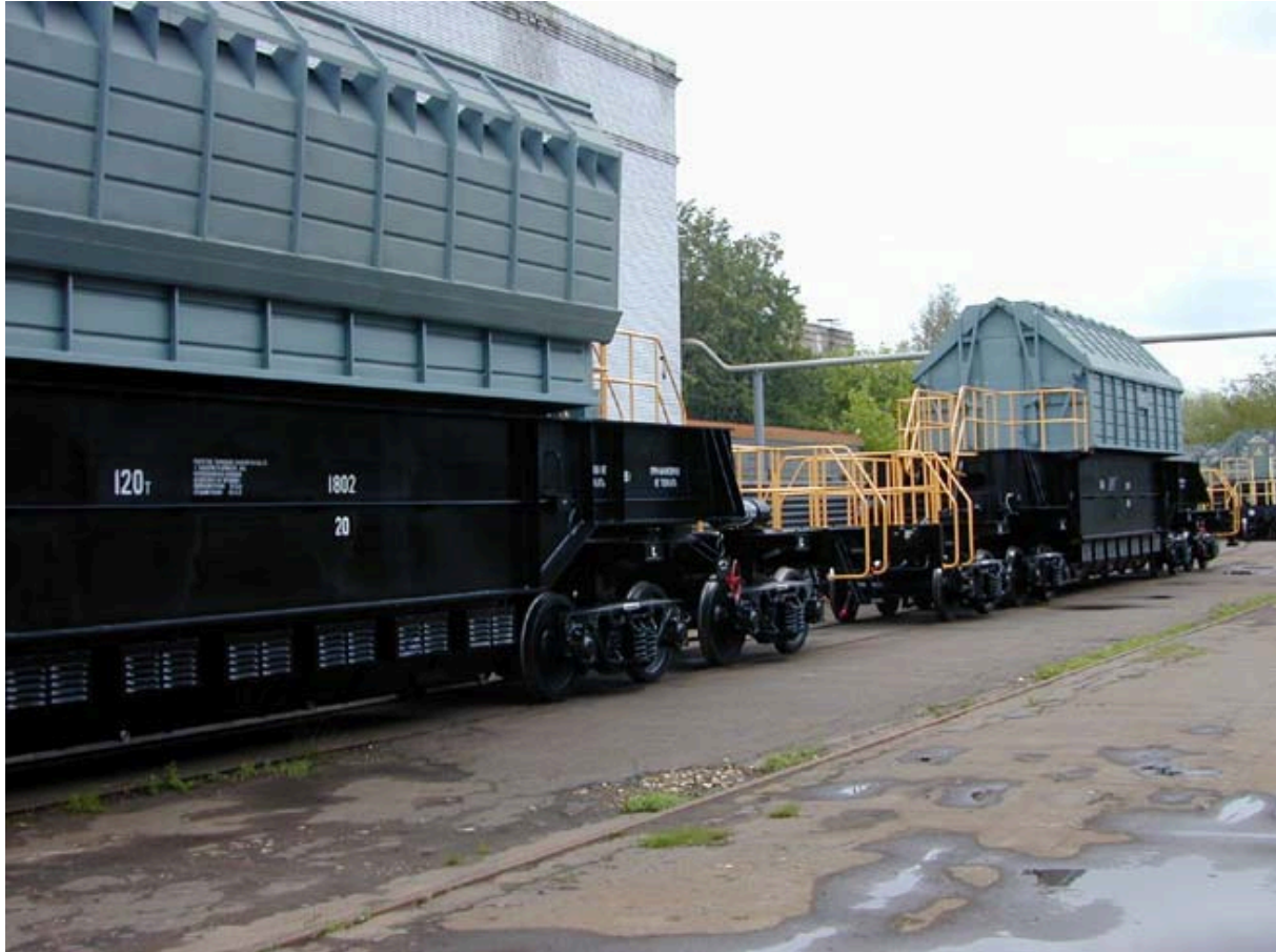
Rail cars for spent nuclear fuel transportation designed and manufactured under Norwegian assistance to Russia (courtesy of Ministry of Foreign Affairs of Norway)
