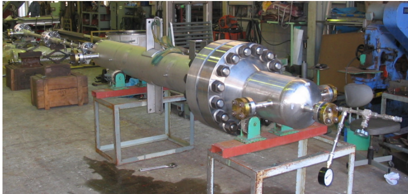
Heater pin bundle, Chimney and Separator
