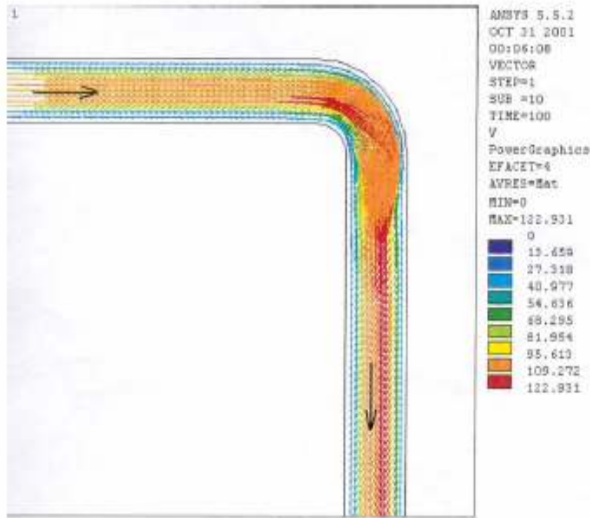
Figures 8. a) 1.8 cm diameter pipe and elbow flow profile with a 0.06 m 3 per minute with a good union and b) The same pipe and elbow with a bad union with a gap of 3 mm. Velocities are in inches per second.
