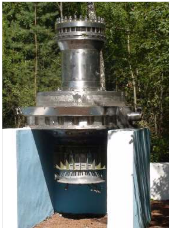
Transportable nuclear reactor designed by SOSNY, Belarus.
