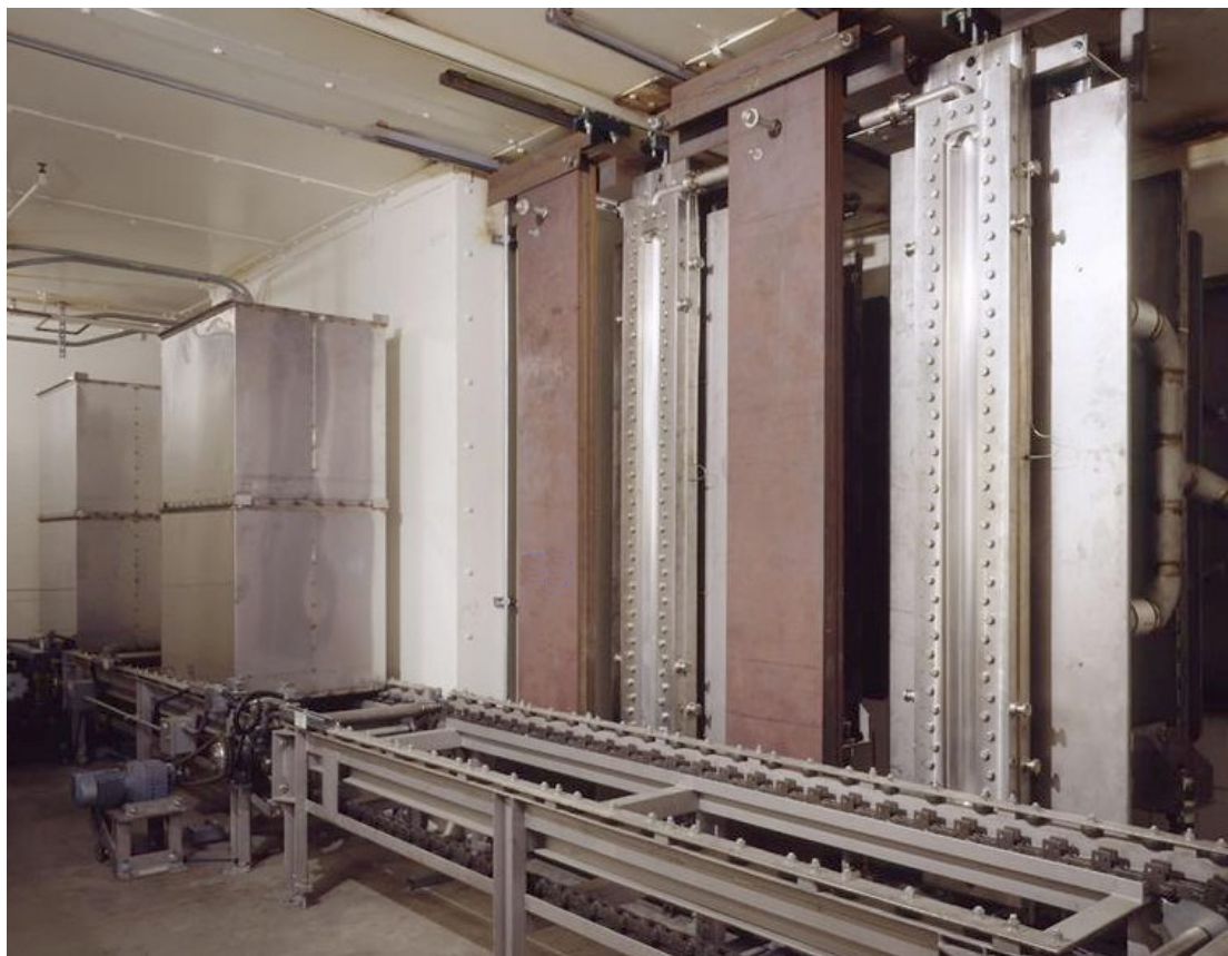
FIG. I-2. Containers with materials (e.g. medical disposables, food products) moving for processing by X-rays from 5–7.5 MeV electron beams.
