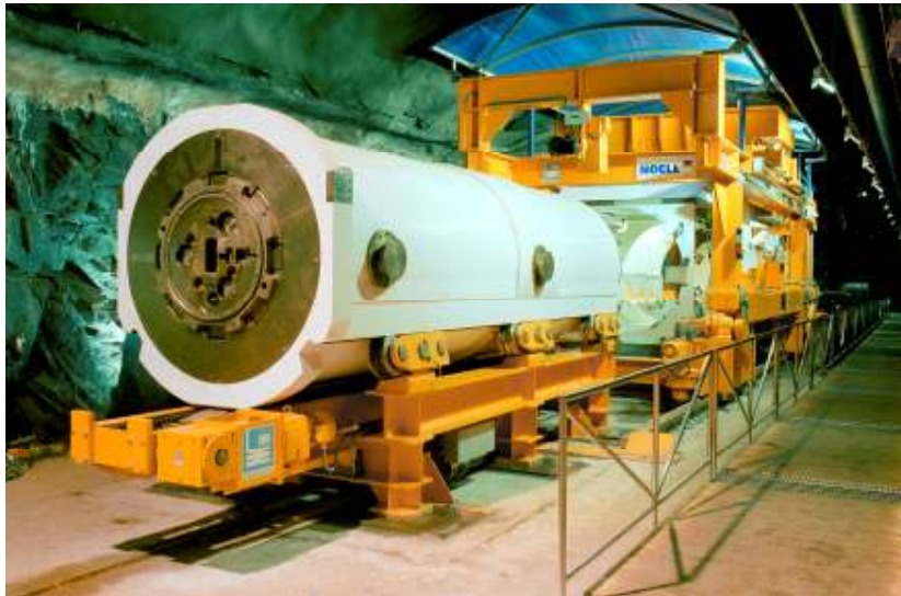
Figure 6. Prototype deposition machine for vertical disposal. The machine tilts the canister into the deposition hole.
